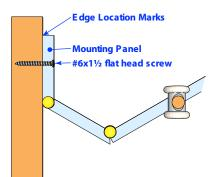
Insert #6 x 1½" flat head screws about 8" up from the floor and 8" down from the track.
