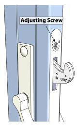
Shut the door, latch it and wiggle the handle a bit. The Latch should swing fully up with the Lead Post pulled snuggly against the Interlocking Jamb Molding.
