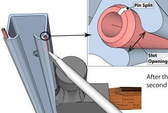
After the track has been secured, drive the alignment pins back halfway into the second piece of track with a hammer and the edge of a screwdriver.
