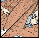
1. Measure a 3" slot, 11/2" each side of ridge centerline. This allows for a 2x ridge board or smaller. Snap chalk lines the entire length of the ridge. Cut slot with a circular saw and clean out debris. Set saw depth so as not to cut roof rafters. Stop the slot 12" short of any ridge end, intersecting ridge or obstruction (such as a chimney).
